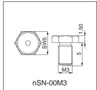
Hydraulic-type lube nipple for sizes 20 and 25
